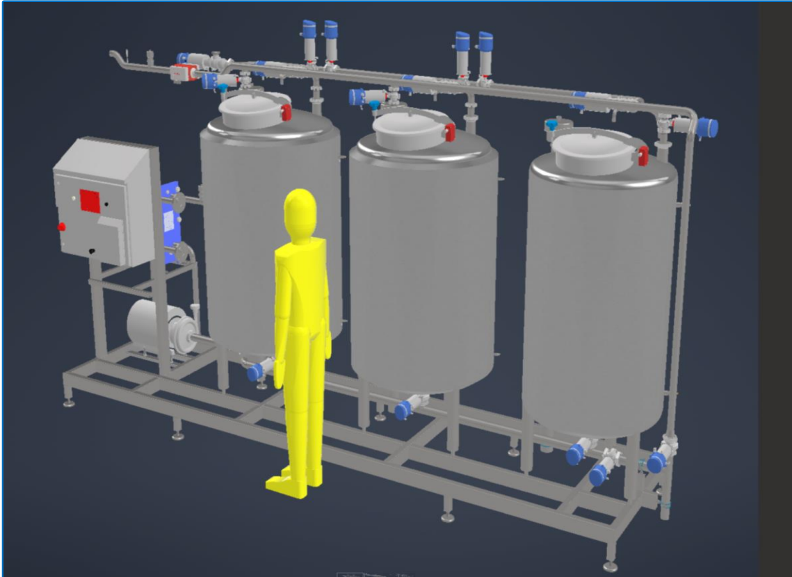
3 Tank CIP set – RHS Final Rinse Tank
